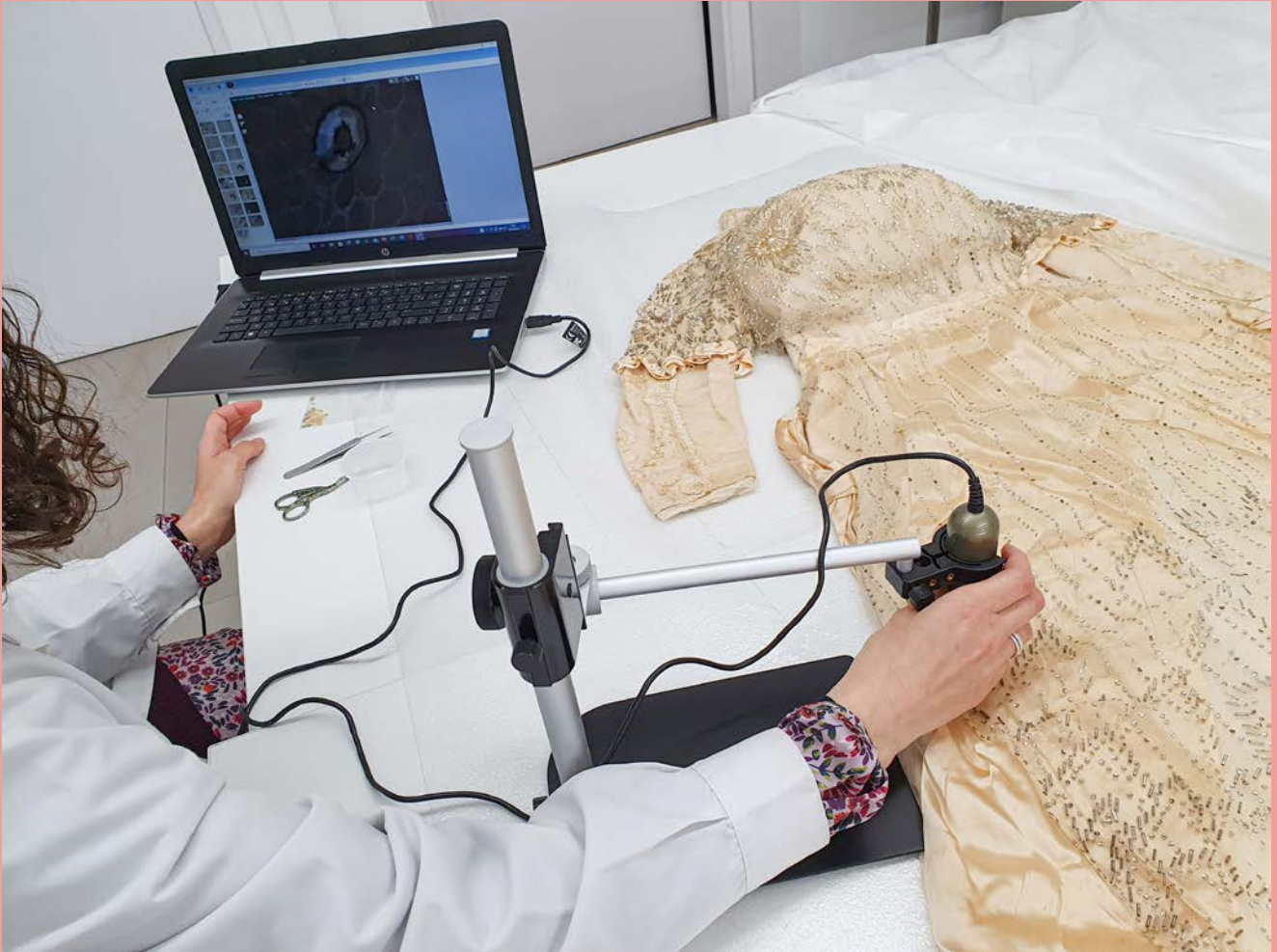
Fig. 3. Example of the documenting process of the condition of the dress. Use of the DinoLite® digital microscope.
